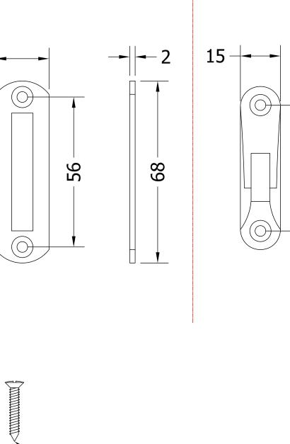
This product is supplied with solid brass woodscrews and one steel screw, the steel screw is intended to be used to cut the thread prior to fixing the door furniture with the brass woodscrews.
