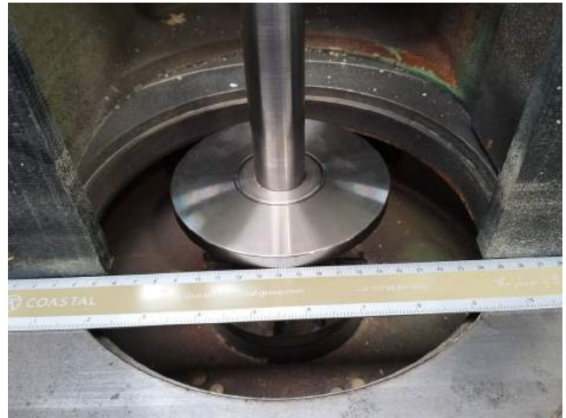
Setting Gauge is then removed and turned over and this becomes the setting point for the fences.
