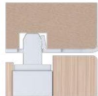
Tritus™ Flush Casement - Pair of sashes lock detail (TOP)
