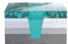
... the substances contained in the nanocapsules repair the resulting scratches and restore corrosion protection.
