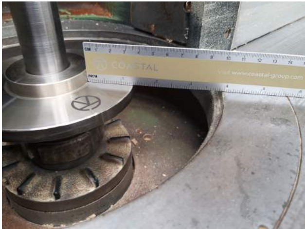
Setting Gauge is placed on the bottom of the spindle shaft with the logo in the up position to determine the bed height as shown above.
