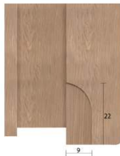
Extra cut-out section on Bottom Sash for friction hinge
