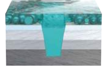
... the substances contained in the nanocapsules repair the resulting scratches and restore corrosion protection.
