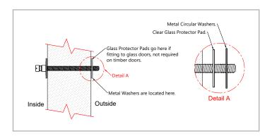
Push the bolt through the hole using the washers provided, if installing on a glass door the Glass Protector Pads must be used first, then the metal washers. If installing on a timber door the Glass Protector Pads are not required, just use the metal washers.
