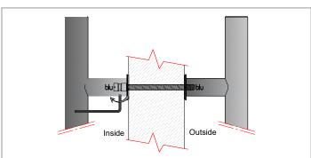
3. Locate the internal handle with the grub screws over the locating pegs both top and bottom simultaneously, push the handle until it is flush with the metal washers. Apply slight pushing pressure then tighten the grub screws hand tight, both top and bottom screws need tightening, the handle is now fitted.
