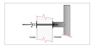
2. Taking the Pull handle without the grub screw, locate the bolt to the hole in the handle and tighten until tight, you can use a screw driver to do this, do NOT use a battery operated driver as this may damage the threads. Repeat this for both holes.
