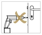
Do NOT use an impact driver, auto screwdriver or cordless or drill to tighten the fixing screw as this can cause the cylinder to bend and not function correctly.
