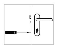
Secure locking cylinder with cylinder fixing screw using a manual screwdriver (max. tightening torque 5Nm).
