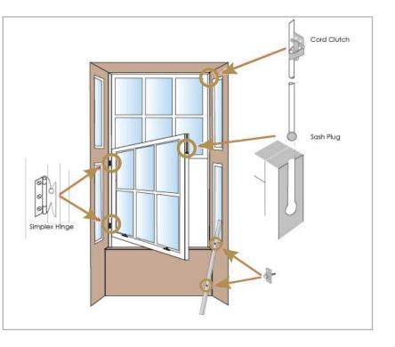
Remove the sash cord from the bottom sash (do not allow the sash cord to suddenly be released as the weights inside the case will drop and may pull the sash cord through the pulley and into the case) and fit a cord clutch just below the pulley for the bottom sash on the face of the case, feed the cord through the cord clutch.
