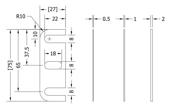
HQ-305-R-SSS - 0.5mm thick HQ-310-R-SSS - 1.0mm thick HQ-320-R-SSS - 2.0mm thick
