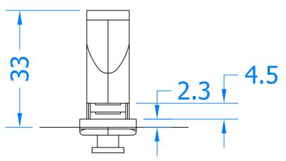
The lock case depth should be 33mm when using the 22mm backset espag.
