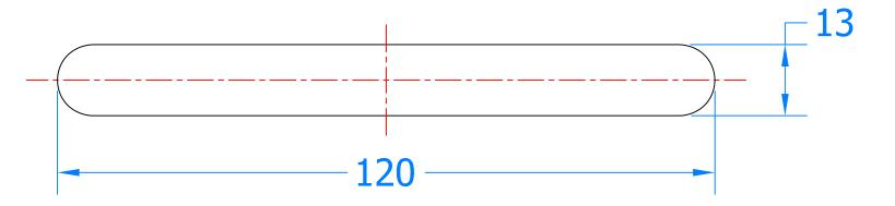
Machine a 13mm wide 120mm long slot centrally to the eurogroove with a 12mm diameter cutter.
