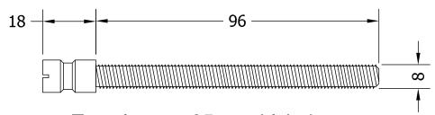
To suit up to 85mm thick doors. 2 x M8 Fixing Bolts
