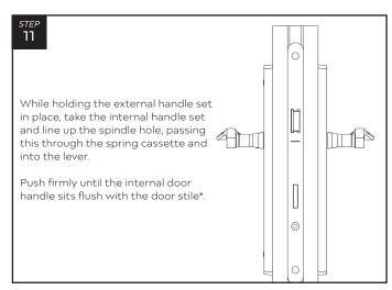
\* If the spindle and threaded bars are too long, preventing the internal handle set from sitting flush to the door, shorten by cutting the spindle.
