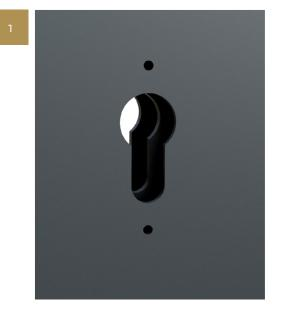
Machine out the Euro Profile cylinder cut out, also drill 2 x 2.5mm holes 15mm deep to accept the screws.
