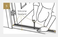
Bed the door sill firmly into place and close the door to re-check for exact positioning. Screw down all fixing screws.
