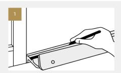
If necessary cut the door sill to the correct length i.e. the exact width of the door frame opening. This will normally be a fraction wider than the door itself.
