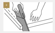
Remove the door from its hinges and saw along a line parallel to the mark and 3mm above it to allow 3mm clearance between the door bottom and the rear upstand of the door sill. Smooth down the sawn surface with sandpaper.
