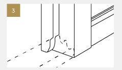
Chisel out sufficient from the bottom of the frame on both sides to receive the front of the door sill, shaping the cut to the profile of the front of the door sill
