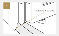
Rehang the door and place door sill in position. Ensure that the door opens and closes freely, the front face of the door butts up to the front seal of the door sill all along its length and the door bottom makes contact with the door sill centre seal. Mark through fixing holes for pre-drilling the threshold. If the threshold is not of wood these holes will have to be plugged to accept the screw.
