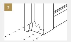
Chisel out sufficient from the bottom of the frame on both sides to receive the front of the door sill, shaping the cut to the profile of the front of the door sill
