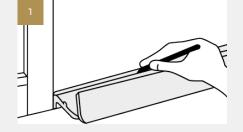
If necessary cut the door sill to the correct length i.e. the exact width of the door frame opening. This will normally be a fraction wider than the door itself.
