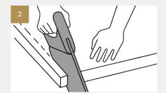
Remove the door from its hinges and saw along a line parallel to the mark and 3mm above it to allow 3mm clearance between the door bottom and the rear upstand of the door sill. Smooth down the sawn surface with sandpaper.
