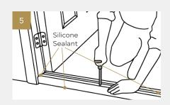
Bed the door sill firmly into place and close the door to re-check for exact positioning. Screw down all fixing screws.
