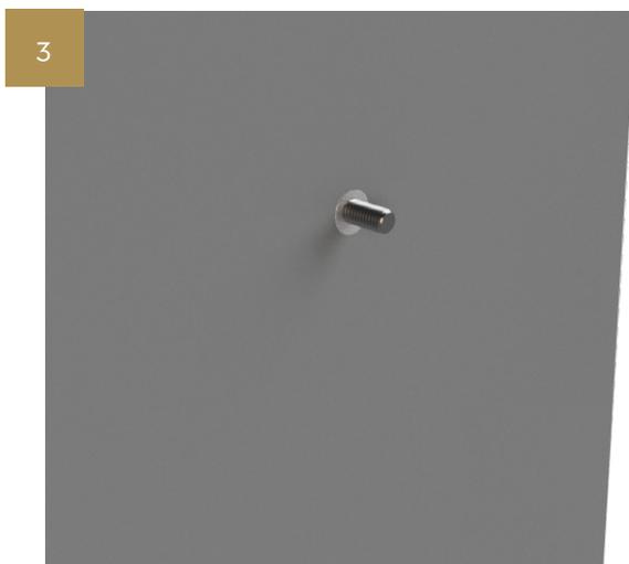
Next screw the threaded bar into the Rampa fixing leaving roughly 15mm protruding.
