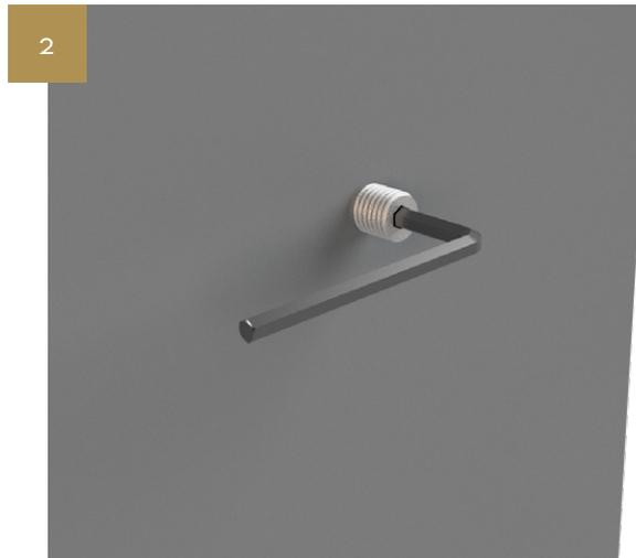
Take the Rampa fixing and locate the small flat end into the hole, taking a 6mm Allen key tighten the Rampa fixing until it is flush to the face of the door.
