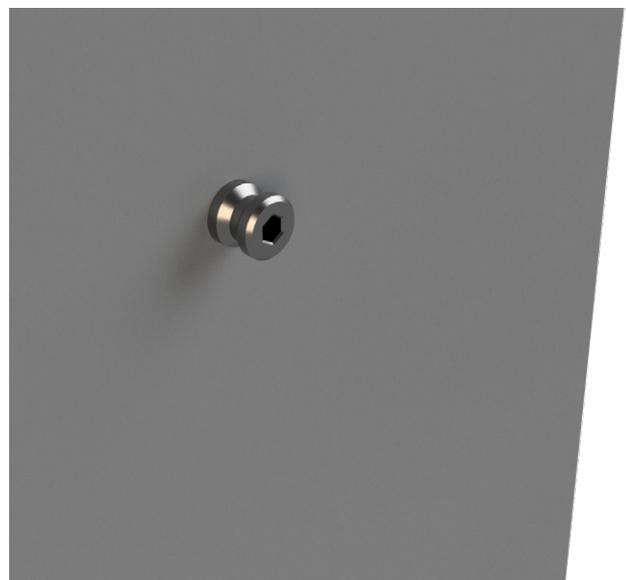
Take the FX-10030-BLU fixing and screw into the aluminium skin using a 6mm Allen key until this sits flush with the face of the door.
