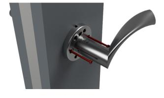
Take the 2 fixing studs (shown in red above) and push them through the 2 outer holes on the external lever, firmly push them in so they are sitting flush with the backplate.
