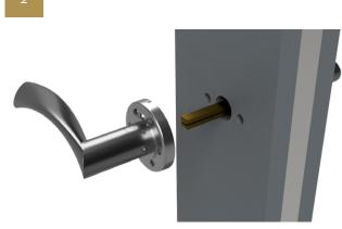
Push the spindle firmly into the internal lever, make sure the grub screw in the lever is wound out to let the spindle pass then slide the spindle through the door lock until the lever is against the door stile.
