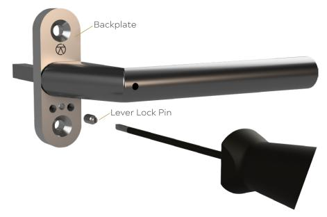
Determine the lever handing, if the lever is for a Right Hand sash then the Lever Lock Pin needs to be installed into the Left-Hand threaded hole in the backplate using a screwdriver.
