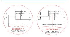
Typical faceplate widths are 16mm or 20mm, this is measured across the face of the lock.
