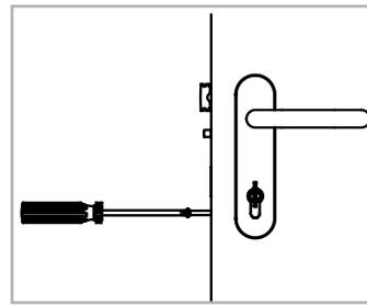
3. Secure locking cylinder with cylinder fixing screw using a manual screwdriver (max. tightening torque 5Nm).
