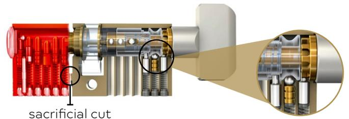
The thumbturn rotor is sprung-loaded, to ensure the cylinder can be operated from the inside in the event of the cylinder being attacked/snapped.
