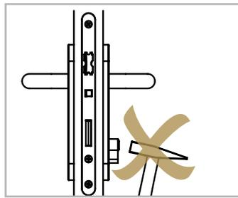
2. Do NOT use force when installing locking cylinder into the lock.
