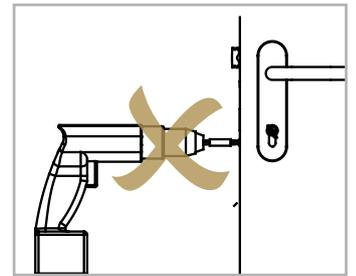
4. Do NOT use an impact driver, auto screwdriver or cordless or drill to tighten the fixing screw as this can cause the cylinder to bend and not function correctly.
