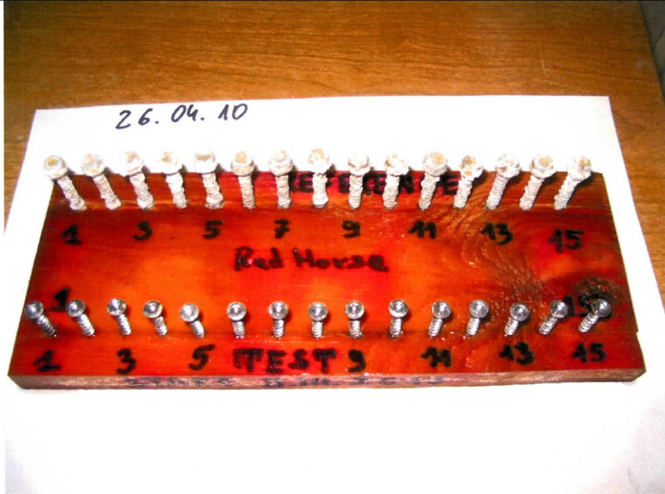
Phot.5. . The screws appearance after 456 hours of salt spray test
