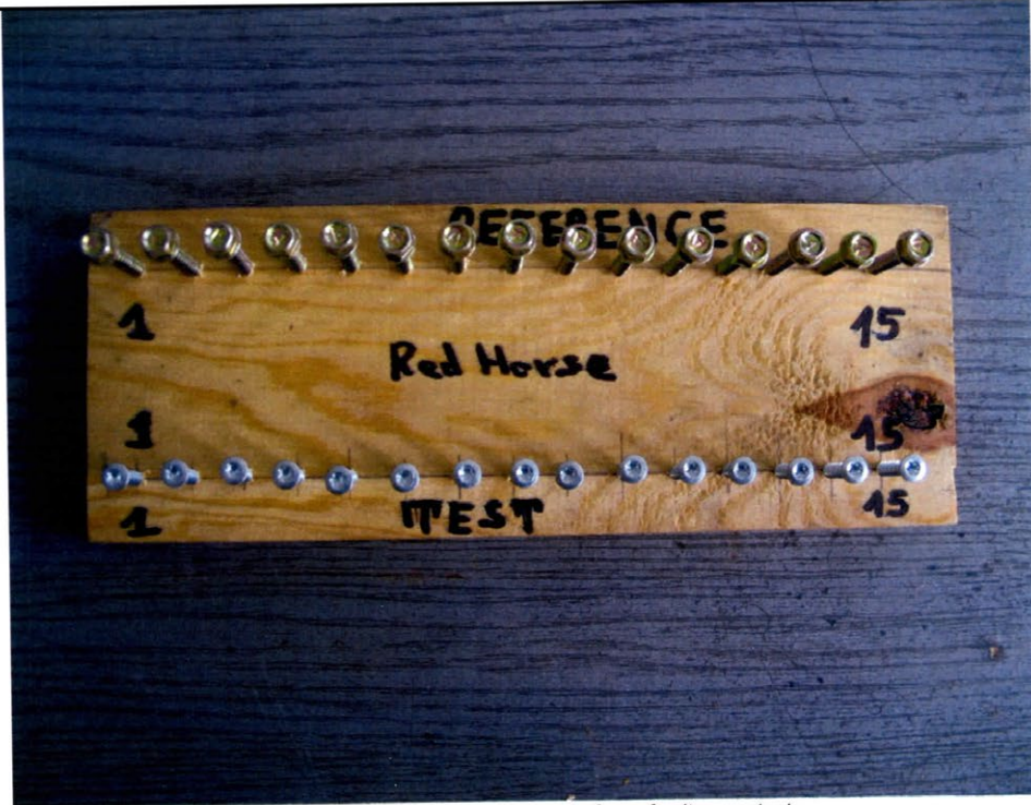
Phot. 1. The screws appearance before of salt spray test.
