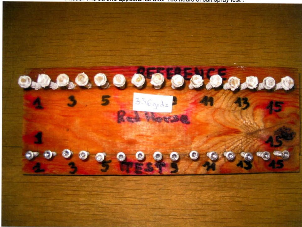
Phot.4. The screws appearance after 336 hours of salt spray test
